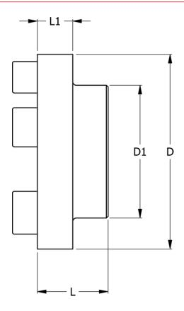
$\begin{array}{lll} D & = 280 \\ D1 & = 180 \\ L & = 110 \\ L1 & = 20 \\ Max bore & = 110 \\ Torque (N m) = 3900 \end{array}$
